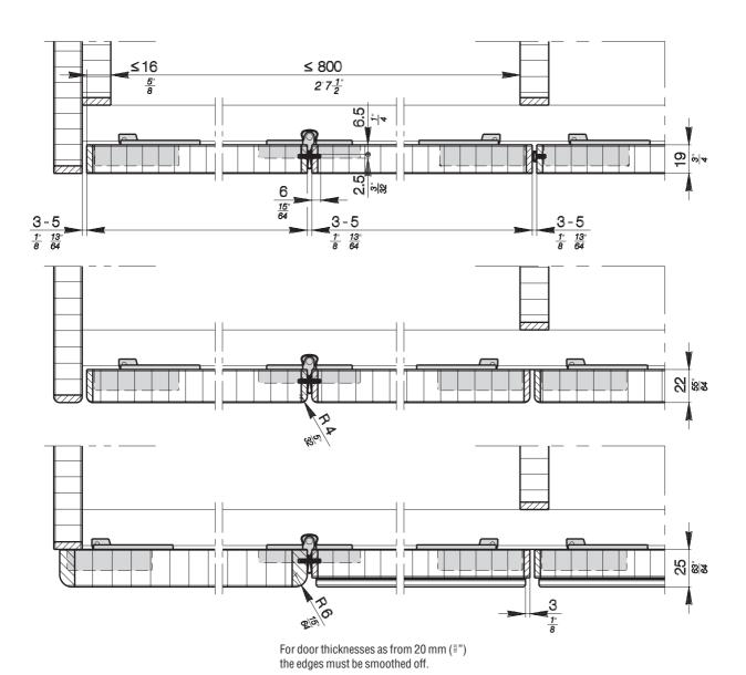
Folding sliding doors provided on one side with 110° concealed hinges with spring.
