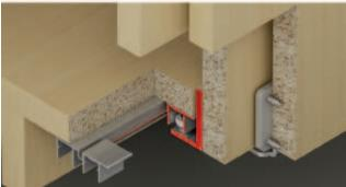
Top running track for groove mounting, bottom roller guide
