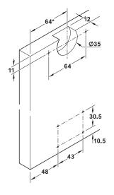
\* = when using inspection support + 64 mm
